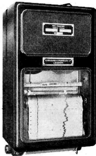
Duplex instrument recording voltage and current on a feeder of an unattended sub-station.
