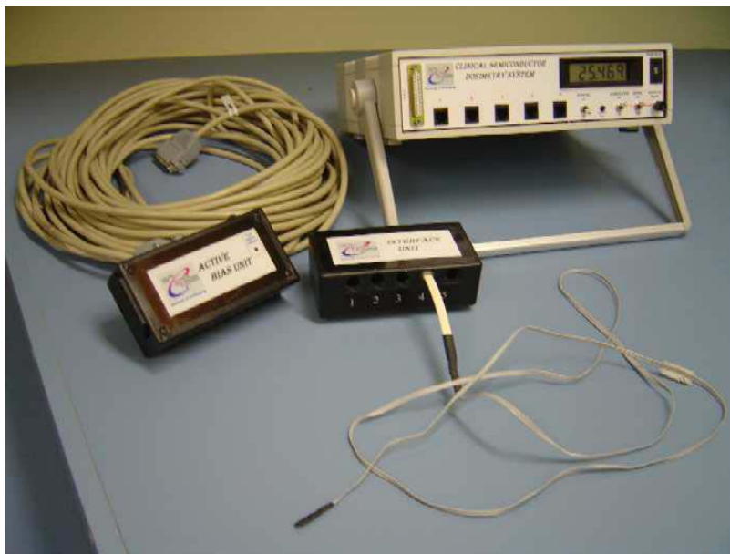
Figure 4.1 MOSFET reader unit with associated hardware. Readings can either be taken on-line via the cable and Interface Unit, or the Active Bias Unit can be used off-line
