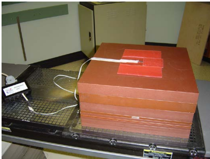
Figure 4.2 Probe in dental wax channel on solid water ® , connected via the Interface Unit to the reader in the console area. (Build-up sheets removed to show the probe placement)
