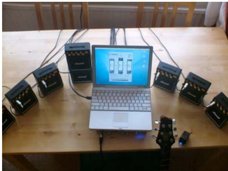
Figure 6.3.2 The ENSEMBLE video game in action with electric guitar, e-bow and the seven agents performing through an array of Marshall MS-2 amplifiers. This system worked with the PowerBook G4, although the later systems require a G5 minimum.
