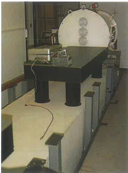
Figure 3.2: Photograph of the pre-isolator slab. The phot also includes the vaccum chamber and the optical table used in the experiment. Equipment seen on the table is seismic monitoring aparatus.
