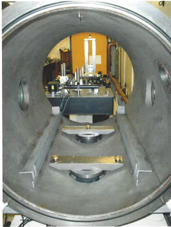
Figure C.1: Photograph of the inside of the vacuum chamber. Isolator feedthroughs can be seen on the floor of the tank. Pumping is through the right port, midway up the side of the tank. The external optical table and suspension tower are visible in the background.
