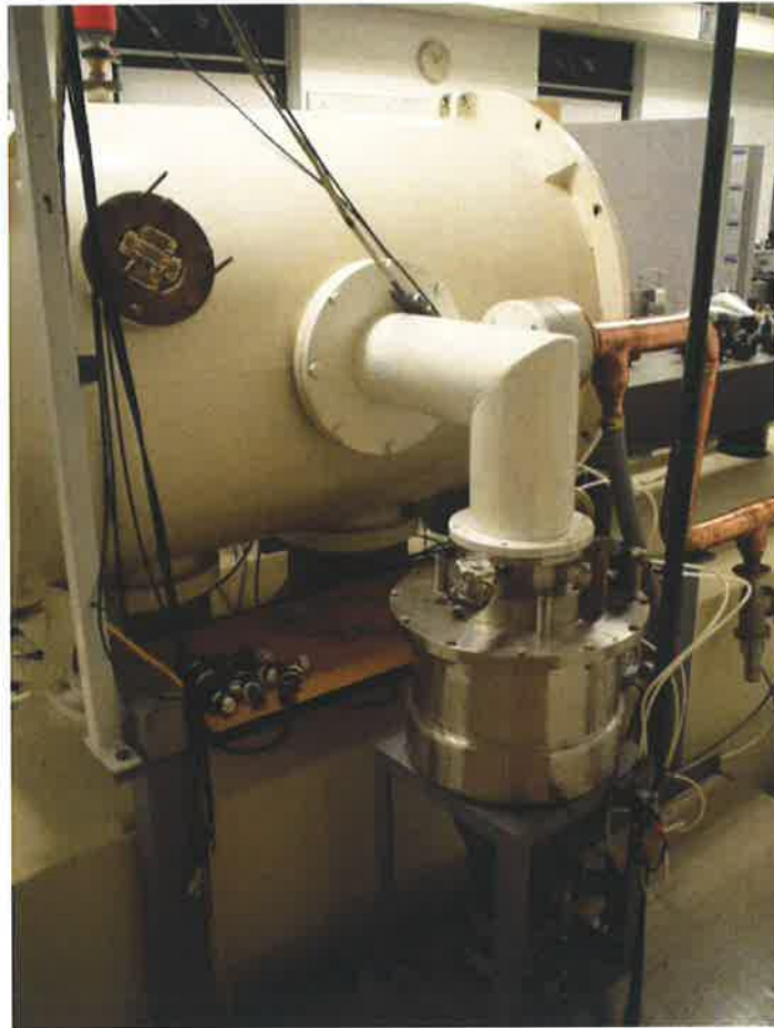
Figure C.5: Photograph of the vacuum chamber, oil trap and diffusion pump. The large silver object in the centre of the frame is the oil trap. The diffusion pump sits beneath it in the grey frame. Both the backing and roughing pumps are attached to the large copper pipe visible in the right of the frame.
