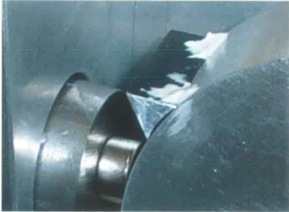
Figure 3.8: Knife edge "ears" mounted on the cylindrical intermediate mass (lower right of picture). White Torr-seal adhesive is clearly visible in the photograph. There is an additional single spot of adhesive on the underside of the ear.
