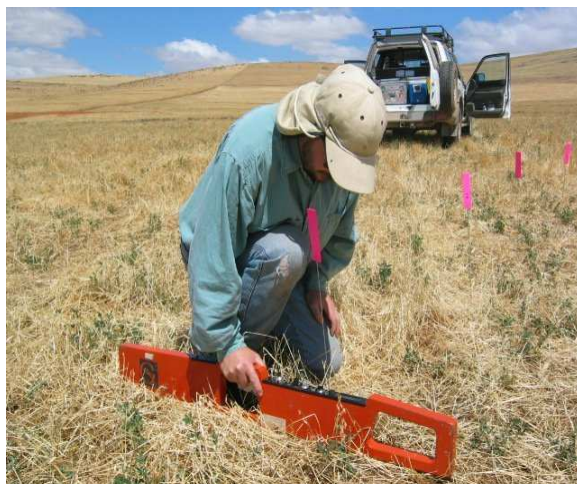
Figure 3.2. The Geonics EM38 instrument in use in vertical mode ( EC_{av} ).
