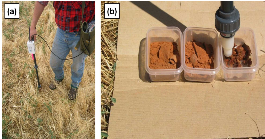
Figure 3.5. Bartington MS2F probe in action. (a) Being used to take measurements from scuffed soil surfaces, and (b) taking measurements of profile samples.
