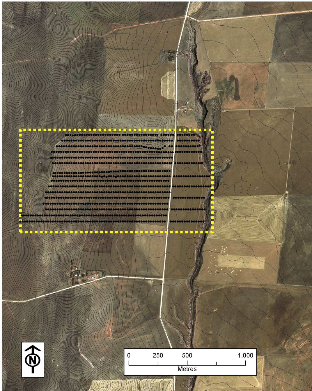
Figure 7.1. Locations of shared geophysical (EM38, EM31 and Bartington MS2D) survey sites (●) of the Midnorth study area.
