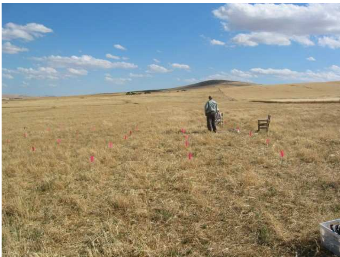
Figure 6.2. Plot survey point marking (pink flags) at 2 m intervals, which are georeferenced using differential geographic information system positioning (photograph of P2 area).
