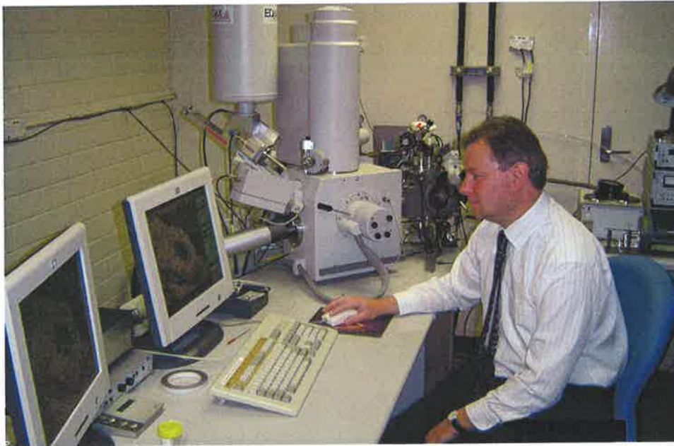
Figure 2.4 The Philips XL30 multi-function microanalytical Scanning Electron Microscope
