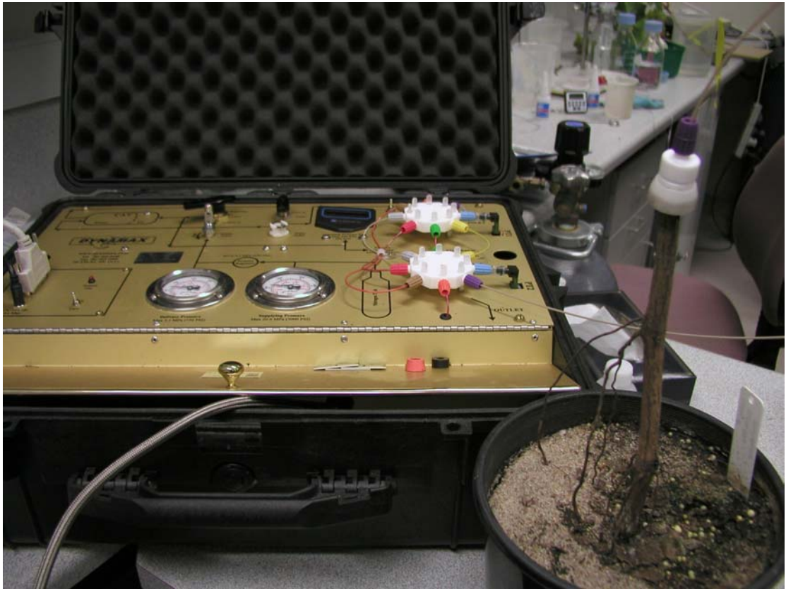
Figure 2.2 Hydraulic Conductance Flow Meter (HCFM) attached to a grapevine stem with the compression fitting.
