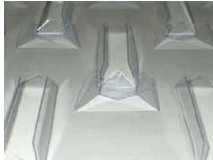
b) Turbulence generator
