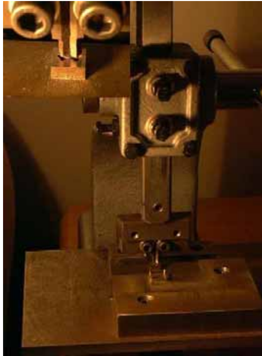
Figure 7.4.1 Photograph of the hand operated punch designed to punch a delta winglet pair, and inset: a close up view of the punch and dye
