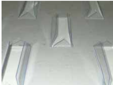
a) Plain fin showing tube holes only
