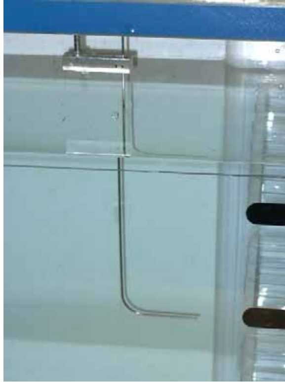
Figure 7.3.2 Photograph of the dye release probe in proximity to the tube bundle located in the flow visualisation water tunnel
