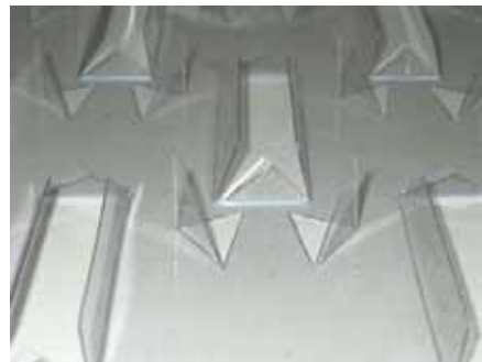
d) Flow Down Vortex generator
