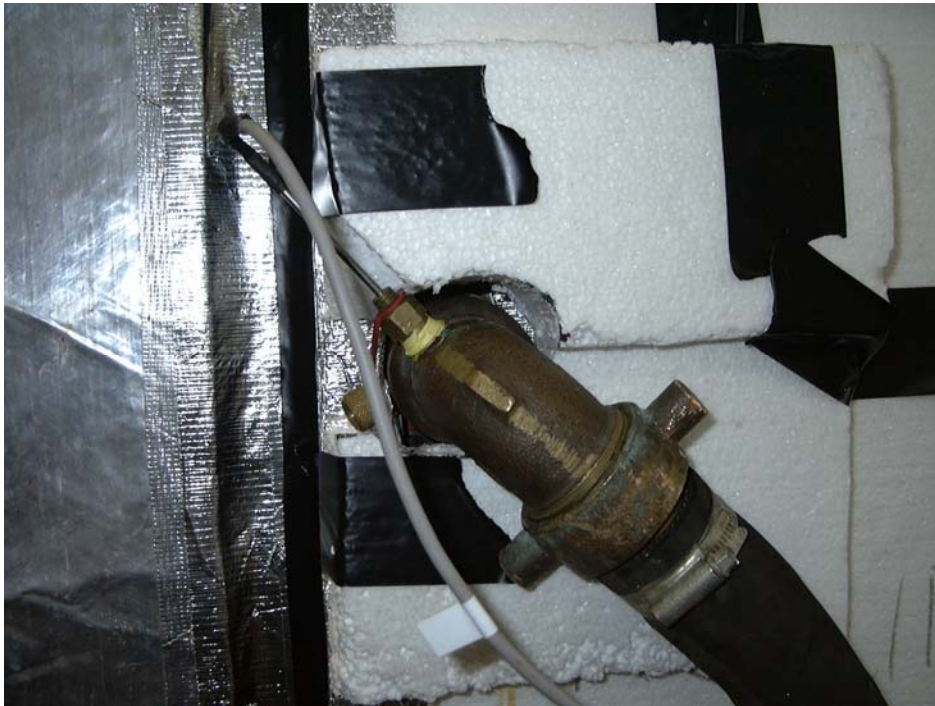
Figure 3.2.2 Photograph showing the location of the PT100 water temperature thermometers
