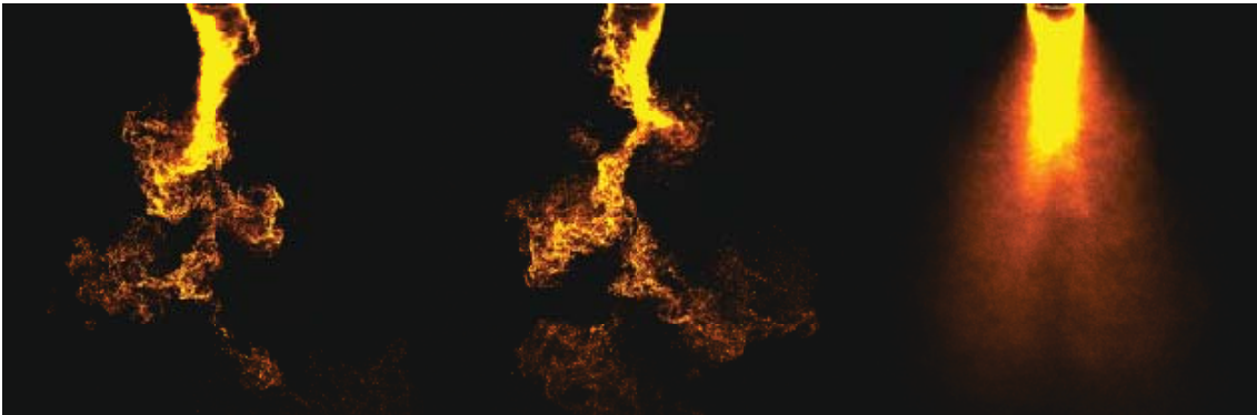
Figure 6.3: Two instantaneous and one mean image of particle distributions emerging from a Precessing Jet nozzle.
