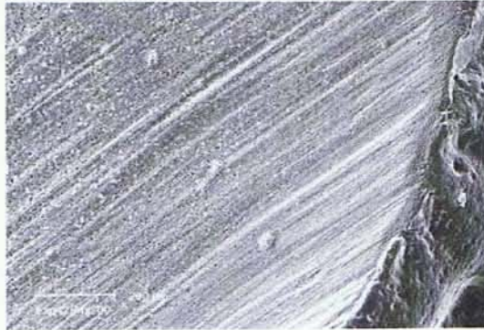
Fig 5. SEM micrograph of an epoxy replica of a dentine specimen in group C worn at load = 100 N and pH = 6.1, but without Tooth Mousse application, after 75 000 wear cycles (x200). Note the very rough surface, with marked striations.
