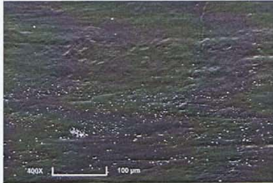
Fig 2. A micrograph showing evidence of abrasion within an NCCL characterized by presence of parallel horizontal scratch marks ( \times 400 magnification). The white spots are artefacts, produced by scattering of electron beams incident on the irregular surface of the NCCL.
