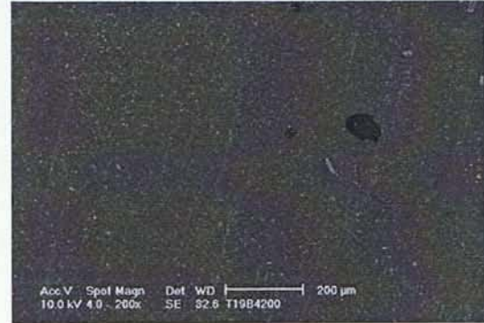
Fig 7. SEM micrograph of an epoxy replica of a dentine specimen in group E worn at load = 100 N and pH = 6.1 after 75 000 wear cycles, with Tooth Mousse applied intermittently (x200). Note the smooth surface compared with Fig 5.
