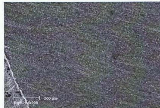
Fig 4. SEM micrograph of an epoxy replica of a dentine specimen in group B worn at load = 100 N and pH = 3.0, but without Tooth Mousse application, after 75 000 wear cycles ( \times 200 ). Note the rough surface with some striations.
