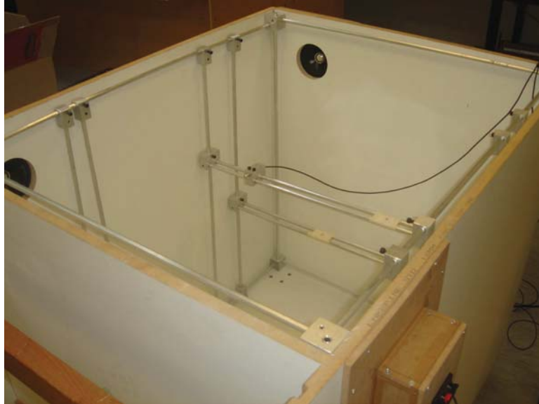
Figure 4.3: The three-dimensional cavity used in real-time experiments. The fixed frame supports the physical microphones.
