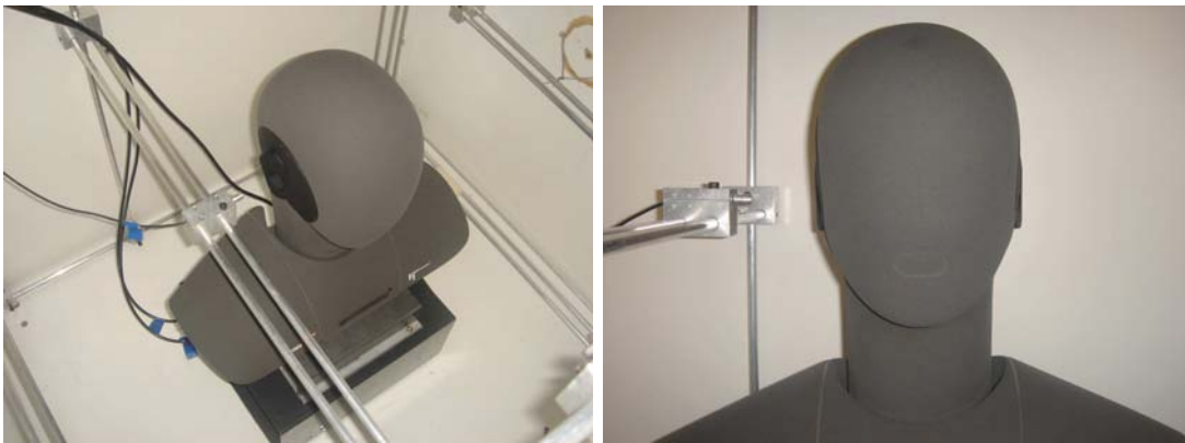
Figure 4.4: The HEAD acoustics HMS III.0 Artificial Head mounted on a turntable and located in the centre of the cavity.
