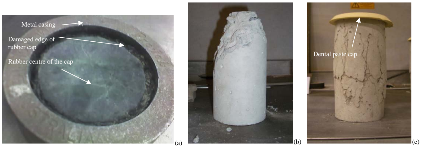
Figure 3-10 Premature failure of early age concrete compression tests.
