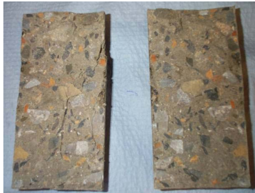
Figure 3-23 An example of a failed specimen from the STS test.
