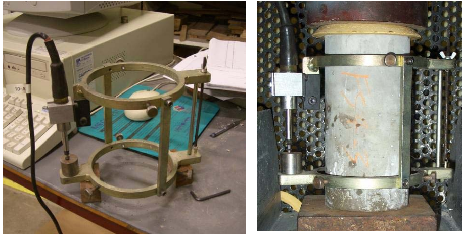
Figure 3-17 Modulus of elasticity two ring test rig.
