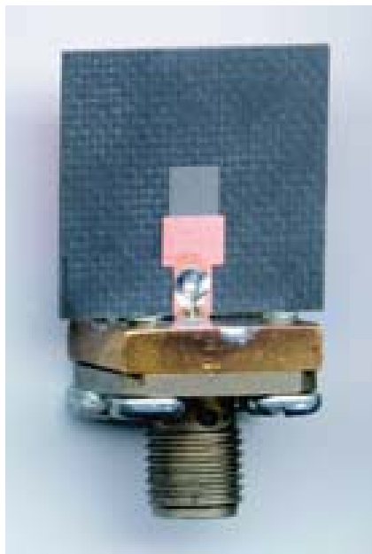
(a) Narrow-band load test structure
