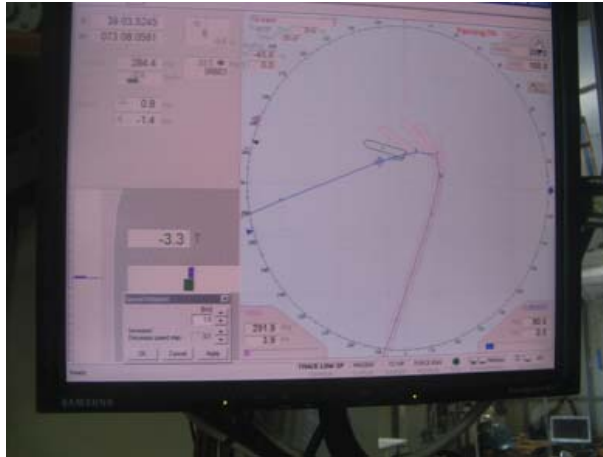
Figure 8.2: Hyperbolic tracks were achieved using dynamic ship positioning. The desired navigation path is entered into the system (blue path) and the actual ship position, shown as grey images, is mapped over time. The ship and navigation path are to scale.
