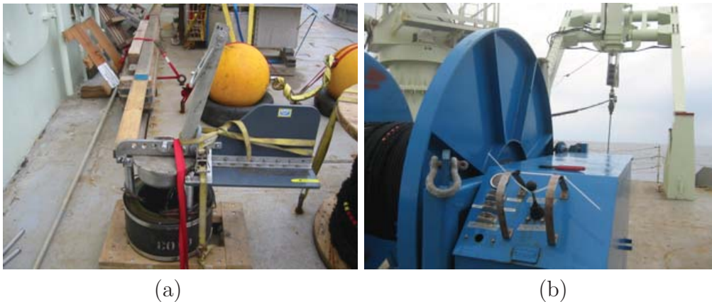
Figure 4.3: Photographs of (a) the ITC-2015 mid-frequency source, and (b) the source being controlled using a ship-board winch (Note the cable ties that were used to control the joystick position, and hence rate of descent, when the source needed to be lowered at a slow but constant rate!).
