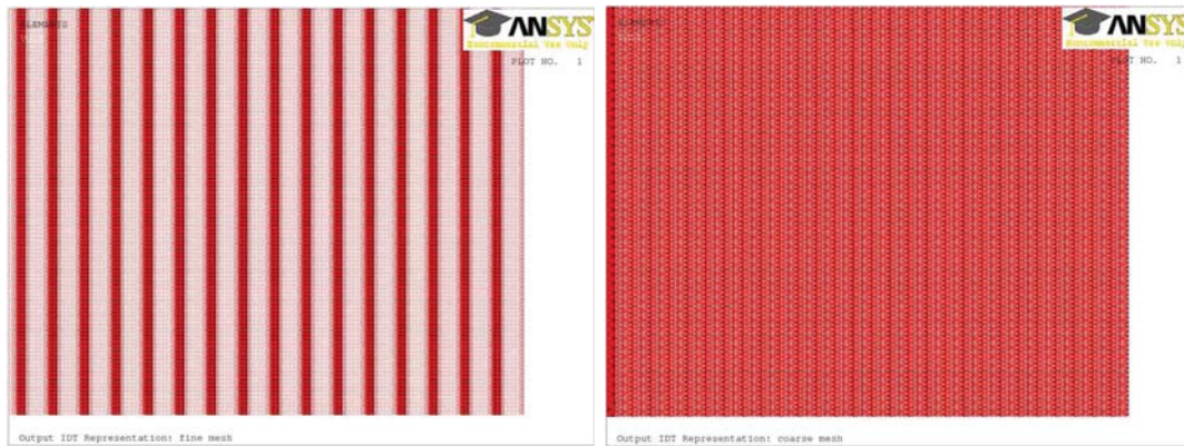
Figure 4.12. Representation of output IDT with different meshes. (a) Output IDT is properly represented in a finely meshed model with an element size of 5 \mu\text{m} . (b) Output IDT is misrepresented in a coarsely meshed model with an element size of 10 \mu\text{m} .
