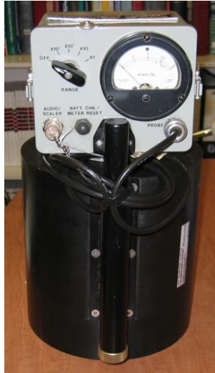
Figure 6.6. A picture of AN/PDR-70 (Snoopy NP-2) portable neutron survey meter (Nuclear Research Corporation, Warrington, Pennsylvania, USA.) used in this study.
