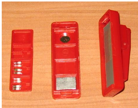
Figure 6.3. (Top) Enriched {}^6\text{LiF:Mg,Cu,P} (clear colour) and {}^7\text{LiF:Mg,Cu,P} (green colour) glass-rod TLDS obtained from Gammasonics Institute for Medical Research, Australia, (Bottom) TLD holder with cadmium filter installed.
