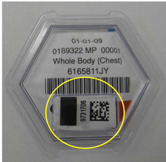
Figure 6.7. A picture of the Landauer® Luxel®+ Ja type dosimeter. This dosimeter is normally used as a personnel dosimeter at the Royal Adelaide Hospital, South Australia. The rectangular part (yellow circle) is the CR-39 etch-track detector used for neutrons measurement.
