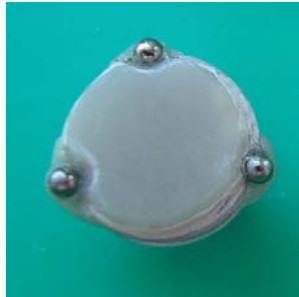
Figure 6. 11: Porcelain specimen on SEM stud with three reference metal balls.
