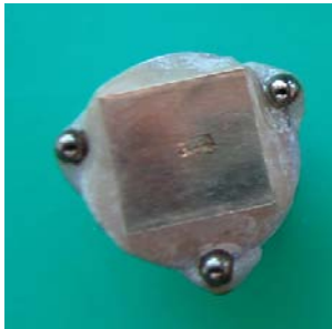
Figure 6. 12: Gold specimen on SEM stud with three reference metal balls.
