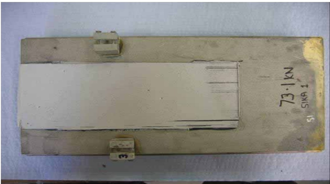
(b) Adhesive layer at failure
