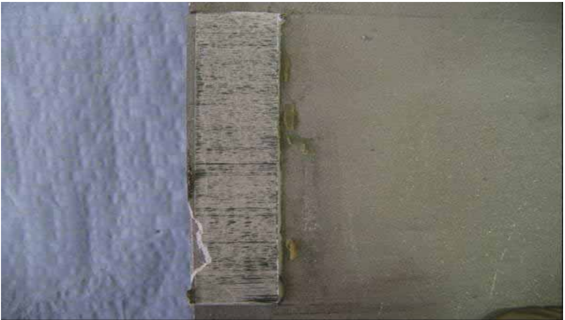
(b) Adhesive layer at failure
