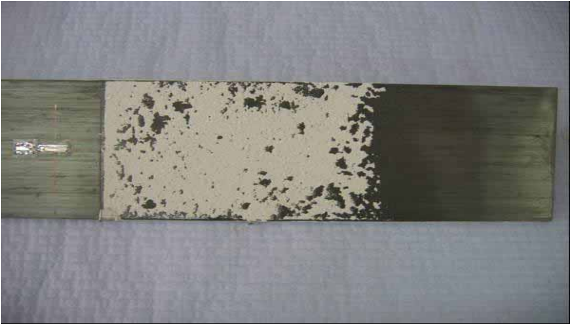
(a) FRP plate at failure
