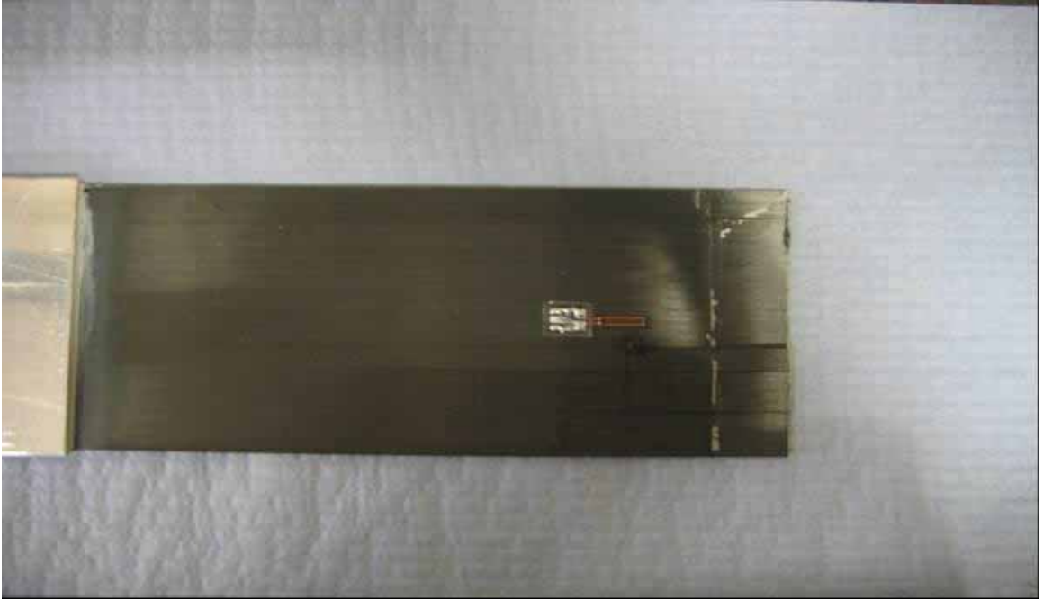
(a) FRP plate at failure
