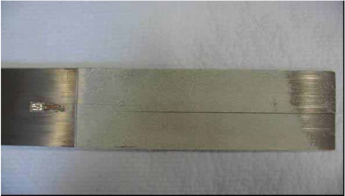
(a) FRP plate at failure
