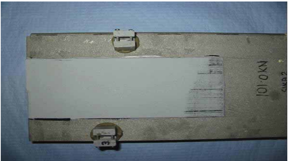
(b) Adhesive layer at failure
