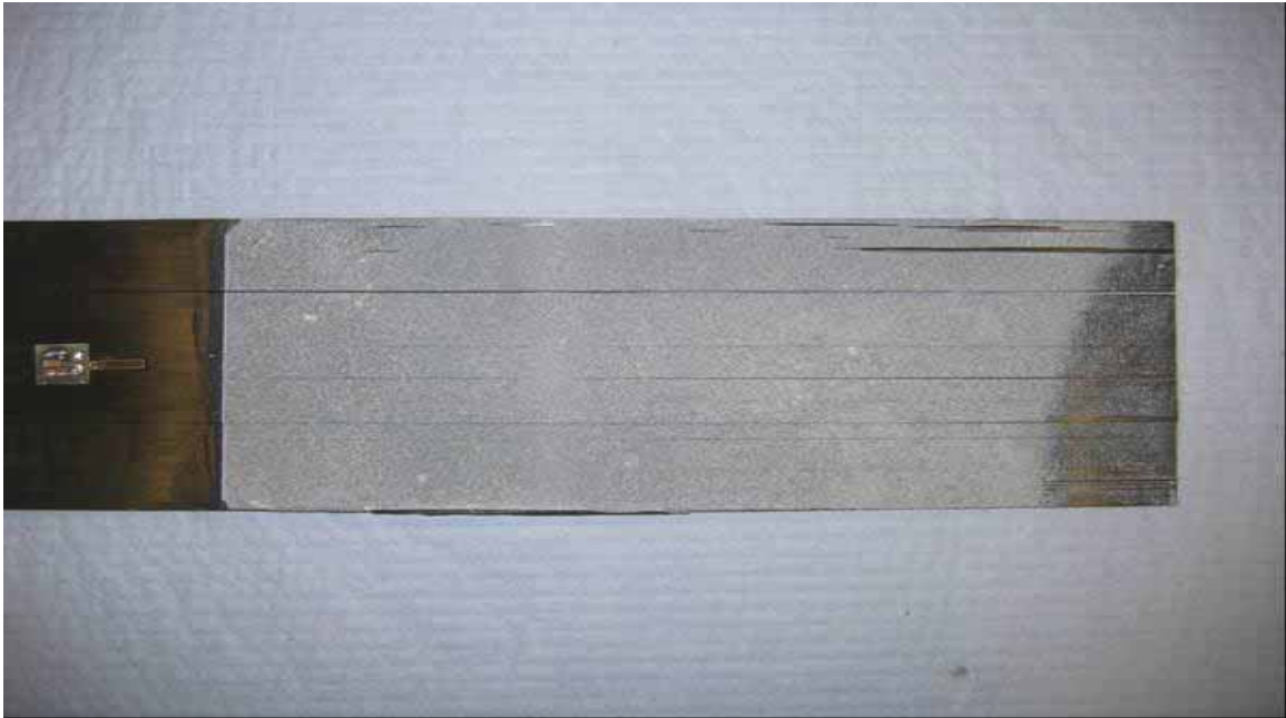
(a) FRP plate at failure
