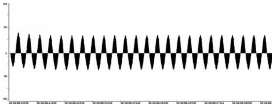
Figure 5: Waveform of a single-operator sinewave when the DAC is at a value of 0.
