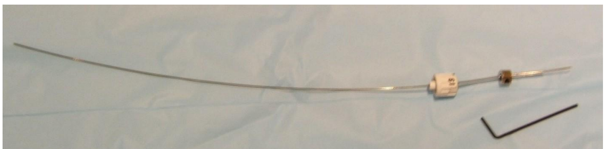
Figure 4-4: Flexible MRI-compatible metal obturator for plastic needles. Length fixed via Leur cap (white) with locking nut on brass clamp tightened onto Teflon tube using allen key.
