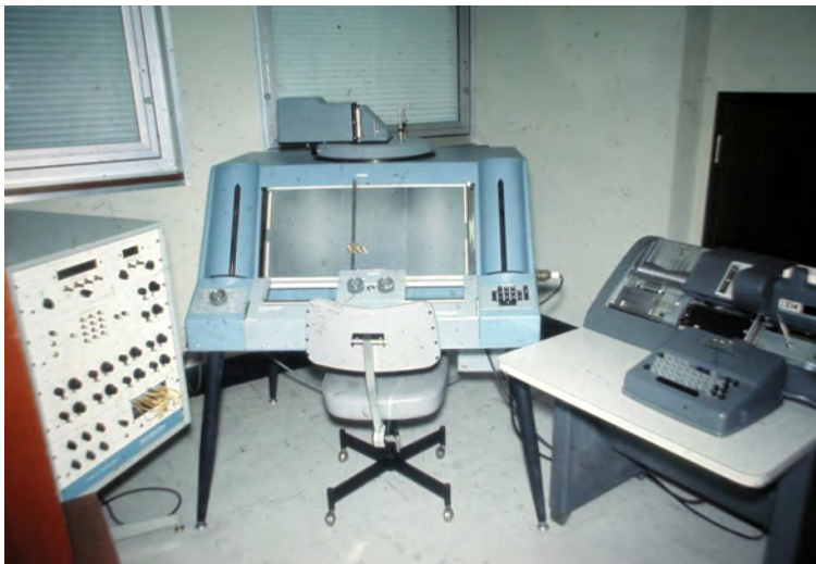
Figure 4.16 OSCAR – the record reader, decimal converter and card punch used to output coordinate data. Manufactured by Computer Industries Inc., Van Nuys, California
