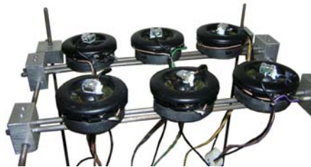
(b) The microphone and speaker array
