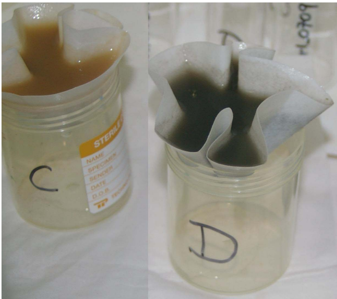
Figure 8-22. Griffith (flask C) and ChangSha (Flask D) soil solutions at day 10 with sulfate addition. Blackened ChangSha soil solution indicates likely presence of sulfide minerals.
