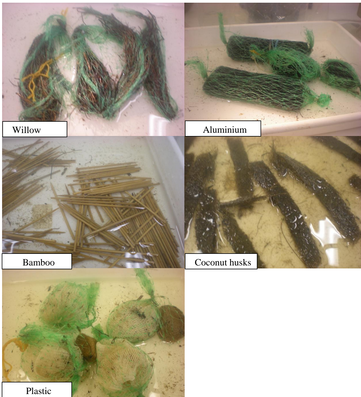
Fig. 1 Photos of five substrate types tested in a trial experiment to compare willow roots and artificial substrates as a habitat for aquatic invertebrates.
