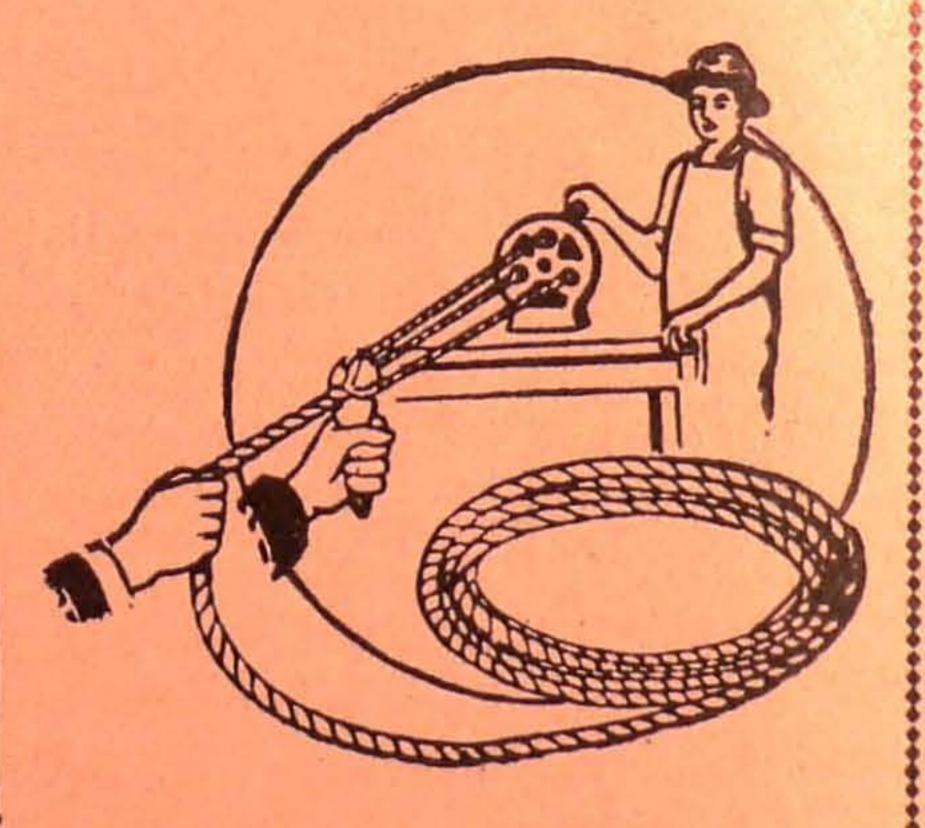
The "New Era" is a great money saver. It enables you to make from binder twine all the rope you need on the farm. Instead of throwing away tangled pieces of twine or allowing odd pieces left over from harvest to dry out and depreciate, you can manufacture them into serviceable rope at a cost FAR BELOW MARKET RATES Write for particulars. Full directions with each machine.
