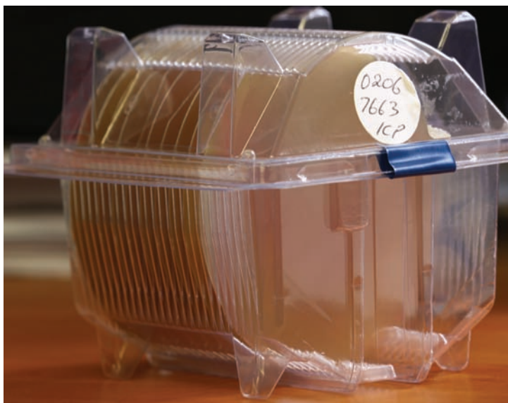
Figure B.3. SOS Wafers. The packaged SOS wafers consist of a thin layer ( 0.6 \mu\text{m} ) of silicon grown on a sapphire wafer ( 0.53 \text{ mm} ). The SOS wafers are from Vally Design Corporation with 100 mm diameter.
