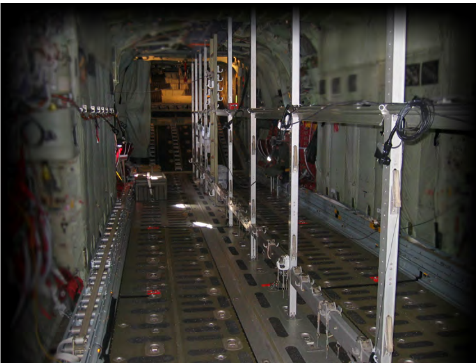
Figure C.13 Main cabin configuration (looking aft), C-130J-30 Trial 2.
