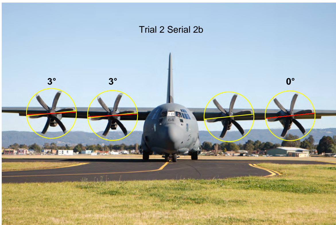
Figure E.3 Ground run photograph from Trial 2 – angles set to (0^\circ, 0^\circ, 0^\circ, 0^\circ) , angles measured as (0^\circ, 0^\circ, 3^\circ, 3^\circ) .
