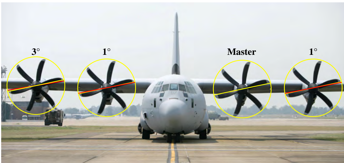
Figure 6.1 Photograph of a C-130J-30 during a ground run with the synchronphase angles set to (0^\circ, 0^\circ, 0^\circ, 0^\circ) and Propeller 2 selected as the master. The angles of the master and slave propellers are represented by the yellow and red lines respectively. The angles measured from this photograph are (1^\circ, 0^\circ, 1^\circ, 3^\circ) . © Commonwealth of Australia. Reproduced with permission from the RAAF.
