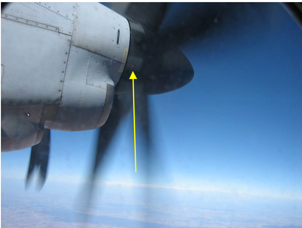
Figure C.9 Laser tachometer aim point, C-130J-30 Trial 1.
