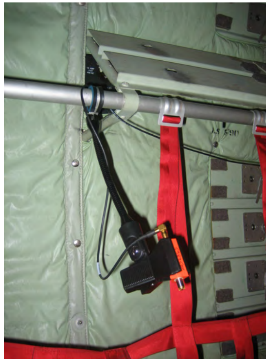
Figure C.7 Typical troop seat microphone installations, C-130J-30 Trial 1.
