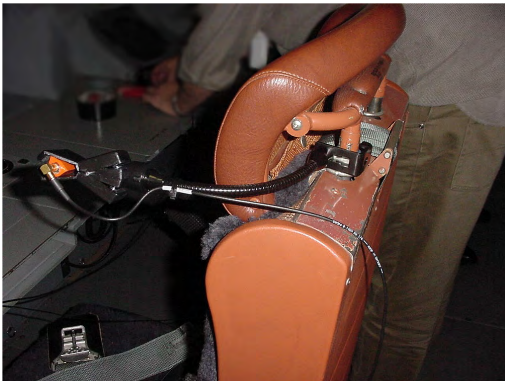
Figure B.2 AP-3C typical crew seat headrest microphone installation on a 20 cm (8 in.) gooseneck.
