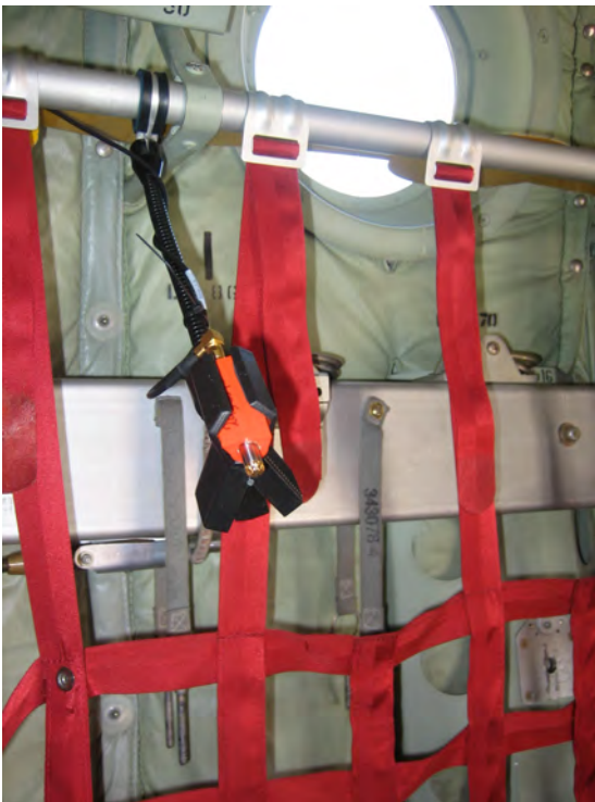
Figure C.7 Typical troop seat microphone installations, C-130J-30 Trial 1.
