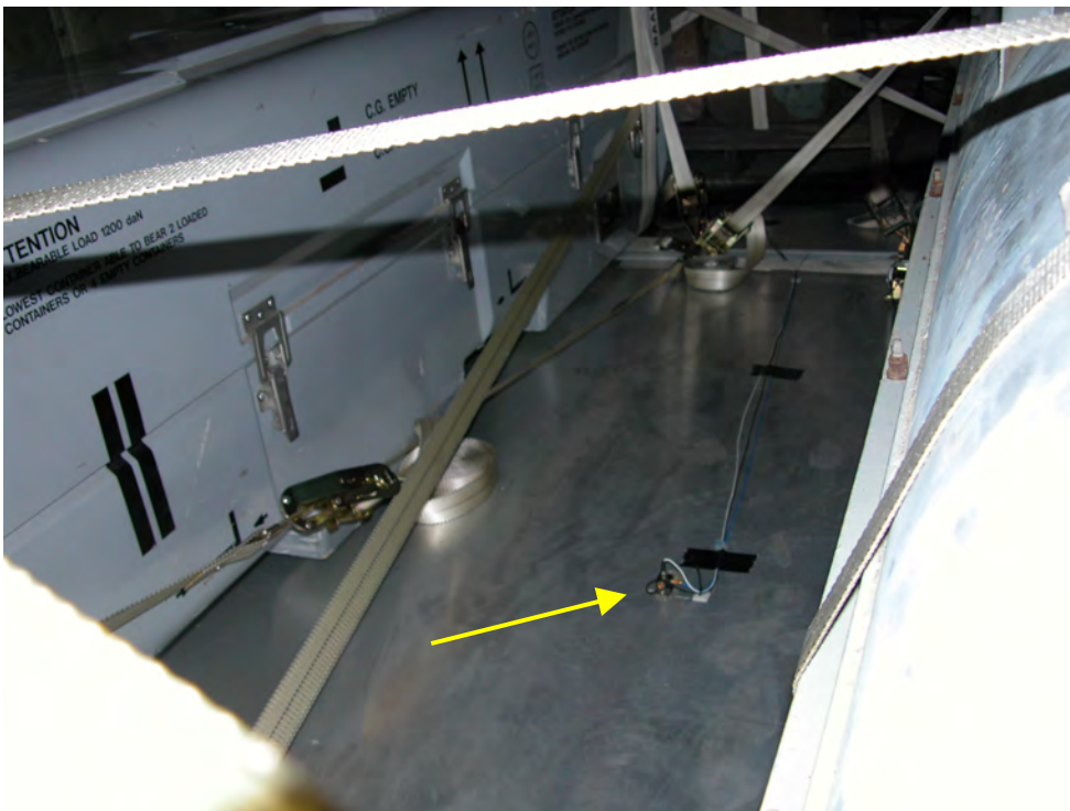
Figure C.5 Tri-axial Accelerometer on the triple pallet (centre of middle pallet), C-130J-30 Trial 1.
