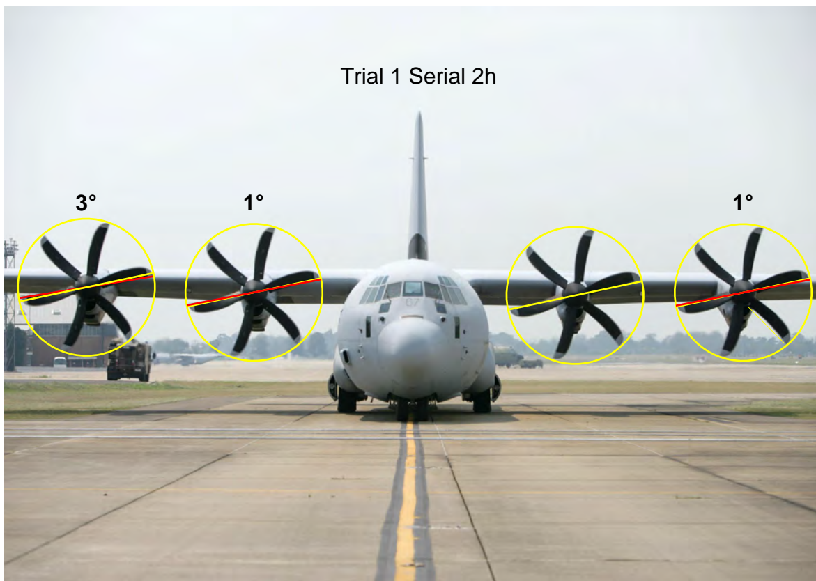
Figure E.2 Ground run photograph from Trial 1 – angles set to (0^\circ, 0^\circ, 0^\circ, 0^\circ) , angles measured as (1^\circ, 0^\circ, 1^\circ, 3^\circ) .
