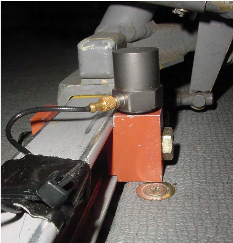
Figure B.3 AP-3C typical seat rail accelerometer installation on a purpose-made bracket bolted through a hole in the seat rail.
