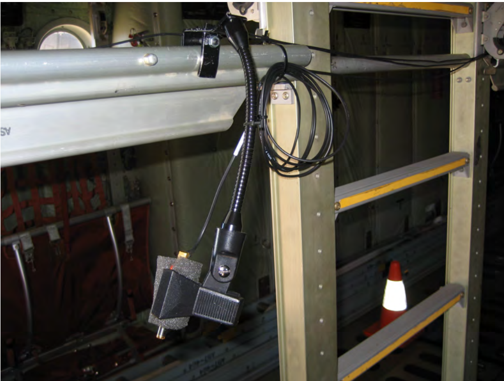
Figure C.16 Microphone mounted to centre troop seat rail, C-130J-30 Trial 2.
