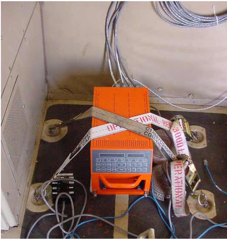
Figure B.5 Heim D120f digital data recorder (hard disk drive removed) strapped to the AP-3C cabin floor.
