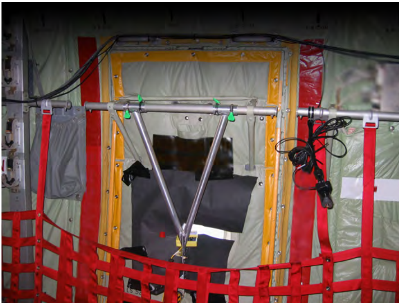
Figure C.18 Laser tachometer (Propeller 1) mounted to troop seat rails, C-130J-30 Trial 2.
