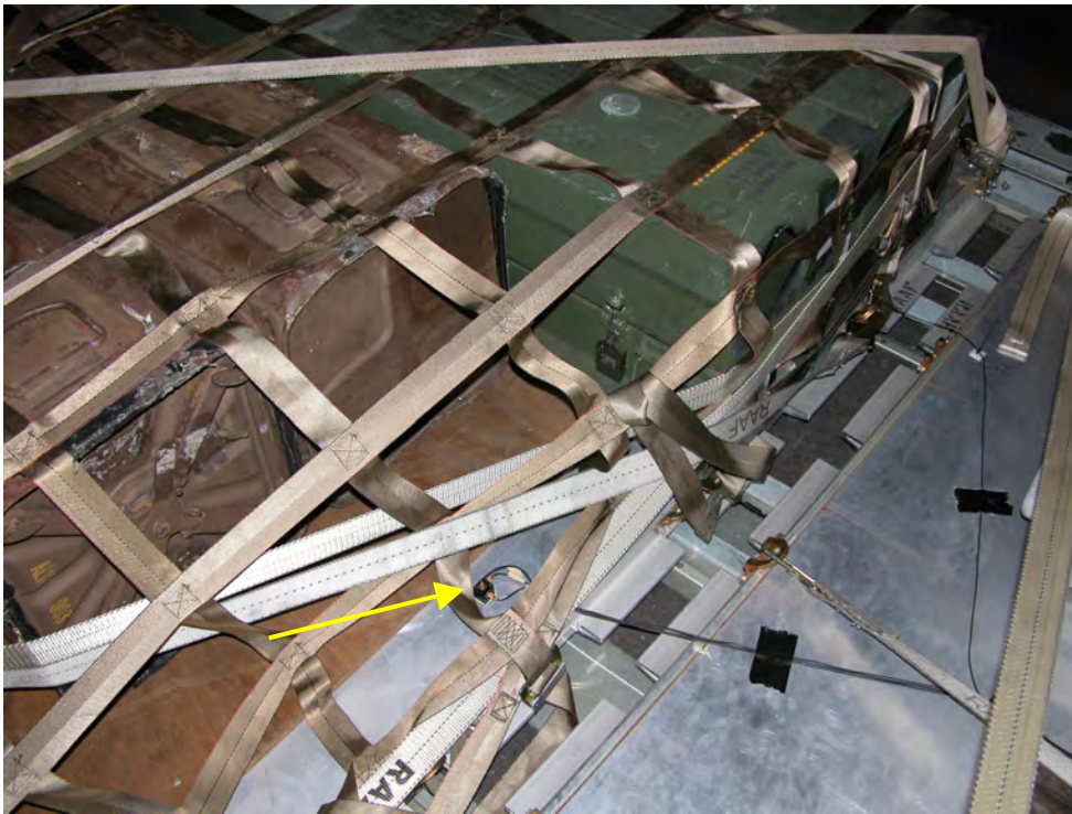
Figure C.4 Tri-axial accelerometer on the single pallet (front), C-130J-30 Trial 1.
