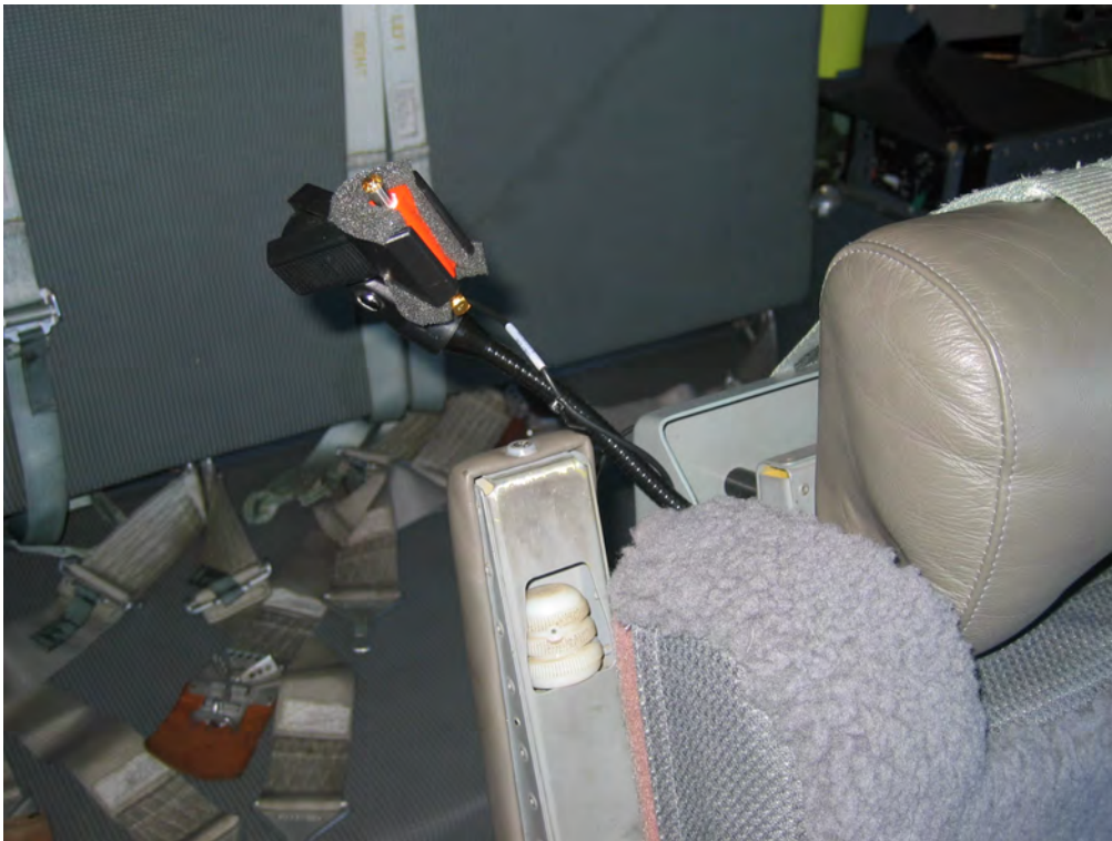
Figure C.14 Microphone mounted to flight deck seat headrest, C-130J-30 Trial 2.
