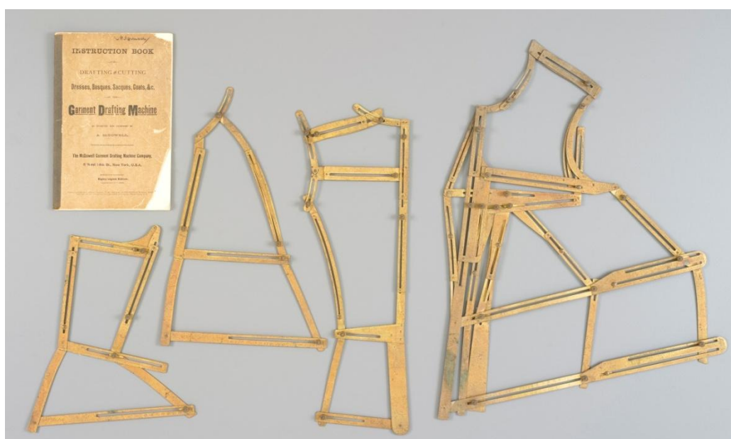
Figure 59: Mc Dowell garment drafting machine and instruction book, (reproduced with permission from Collection: Powerhouse Museum, Sydney. Photo: Sotha Bourn)
