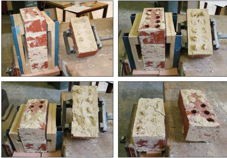
Figure A.4: Typical bond failure of the full-sized perforated brick specimens during bond wrench test.
