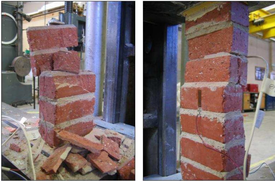
Figure A.16: Typical compressive failure of solid half-sized brick specimens.
