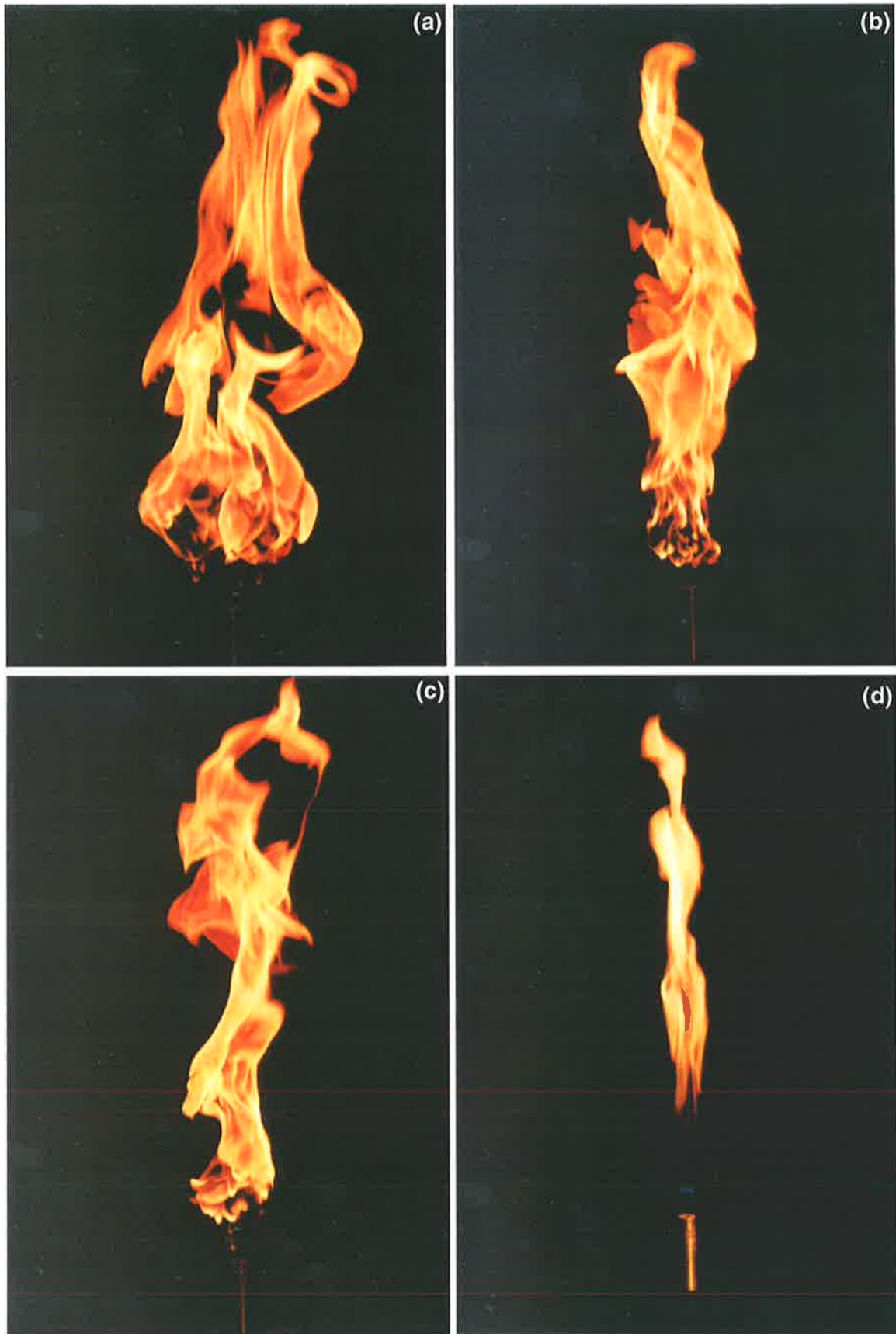
Figure 4-1. Instantaneous images of the visible flame structure from an unconfined PJ nozzle at different proportions of central axial jet to total flow rate. The fuel is propane at a constant input of 20kW, t=1/250 s camera exposure time, f/8 aperture setting. Flow conditions: (a) \psi_{CAJ}=0\% , \Gamma_{CAJ}=0 ; (b) \psi_{CAJ}=30\% , \Gamma_{CAJ}=0.36 ; (c) \psi_{CAJ}=50\% , \Gamma_{CAJ}=0.57 and (d) \psi_{CAJ}=100\% , \Gamma_{CAJ}=1 .
