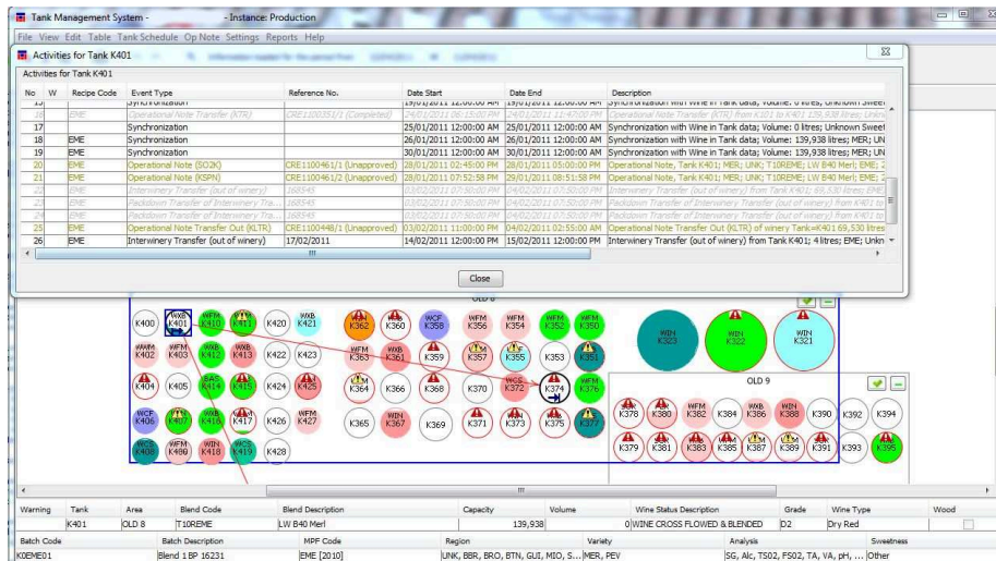
Figure 7.4: Tank Farm Map View Screenshot. The circles represent physical layout and contents (by colour). An Activities popup shows the transactions on a single tank
