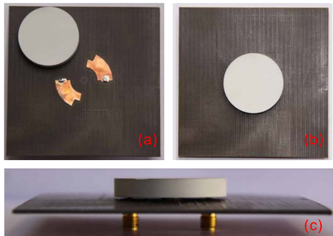
Figure 5.10. Realized prototype of horizontally polarized DRA. (a) and (b) Top view without and with DR on microstrip arcs; (c) Side view.
