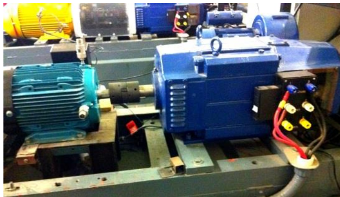
Figure 3.7 Photograph of the experimental setup with the motor under test and dynamometer.
