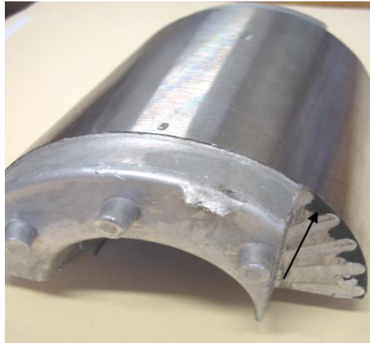
Figure 5.25 The section of the motor used during the test indicating the slot type.
