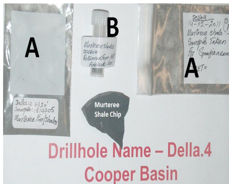
Figure 3.13: Murteree shale (A & B) powder samples in plastic bags used for XRD analyses and small chip before grinding the sample into powder.
