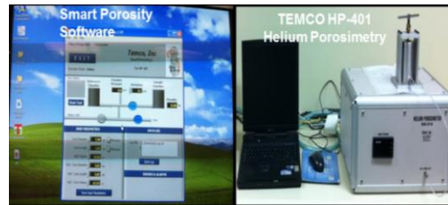
Figure 4.8: Software and TEMCO HP-401 Helium Porosimeter
