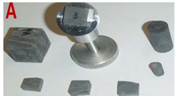
Project Well -Della4 Murteree Shale FIB/SEM Scanned Samples
