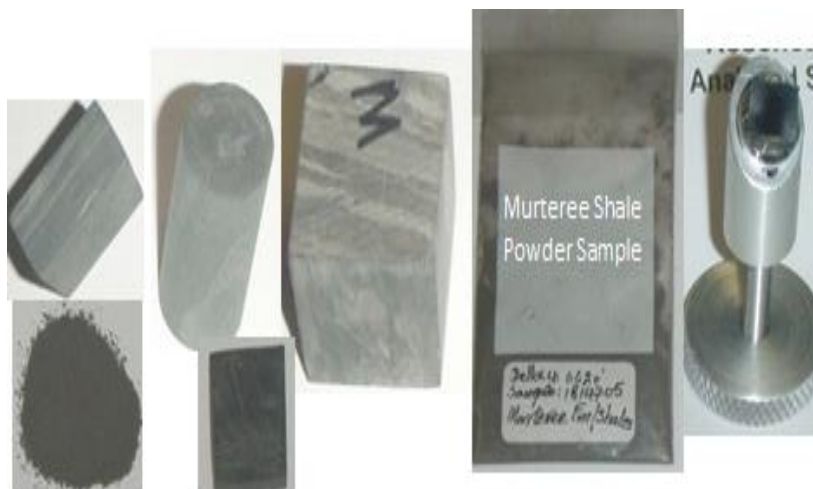
Figure 4.4: Murteree shale samples from project well Della4 used for MICP, Helium Porosimetry, Pycnometry and FIB/SEM Analyses
