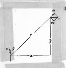
b. The horizontal field due to the vertical component of a dipole.
