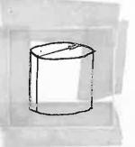
On the specimen is marked a reference line with the aid of which you can determine the original orientation of the rock in the field. This and the
