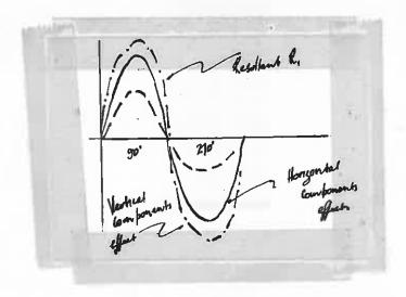
Now if you invert the specimen and again rotate, then in this case the effect of the vertical component is reversed. Of course you must reverse the order of taking readings - the effect of the horizontal field of the horizontal component in the 90° position when the specimen has been inverted is equivalent to it's effect in the 270° position before the inversion took place.
