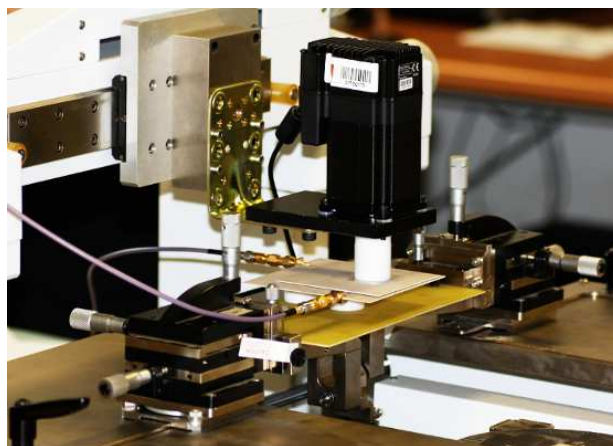
Figure 5.20. Measurement setup for the 2-D displacement sensor. Measurement setup, which is composed of three sets of micrometer actuators for accurate adjustment of the air gap between the substrates as well as displacement in x and y directions. The measurements have been performed at the Laboratory of GEMMA/CIMITEC, Departament d'Enginyeria Electronica, Universitat Autònoma de Barcelona, Spain.
