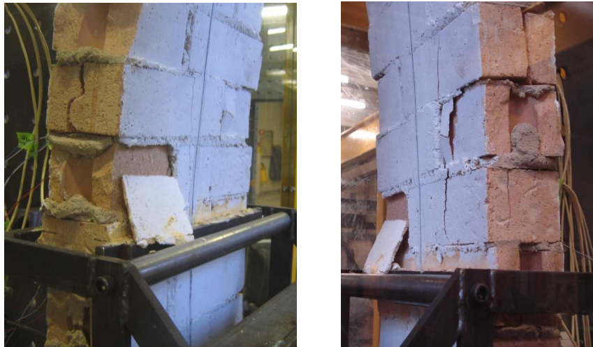
Figure 6-2: Failure on compression face of test specimen
