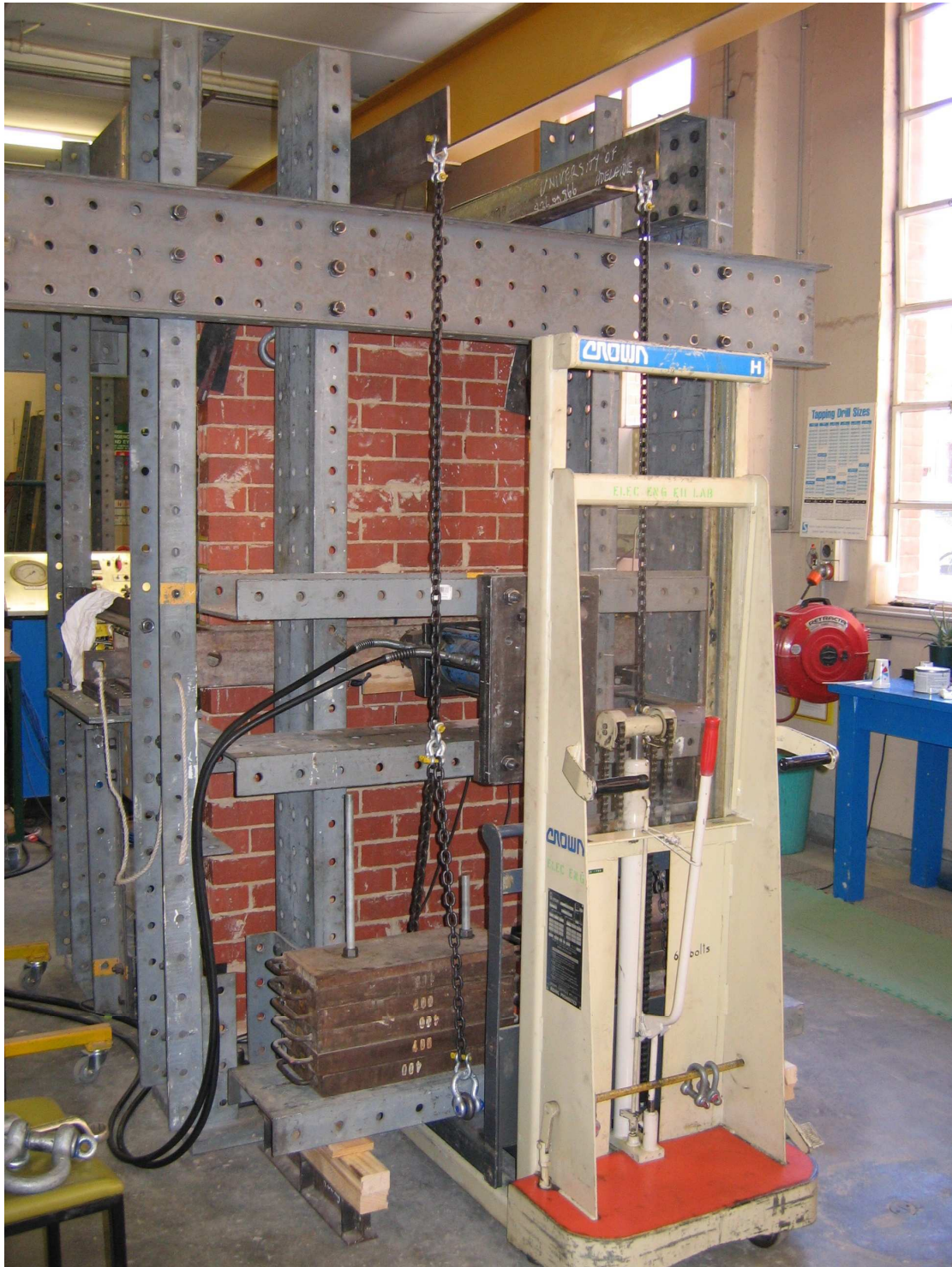
Figure E-4: Axial load set up for wall test
