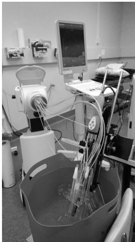
Figure 30. OCP verification experimental setup using a PMMA phantom submersed in a water medium.
