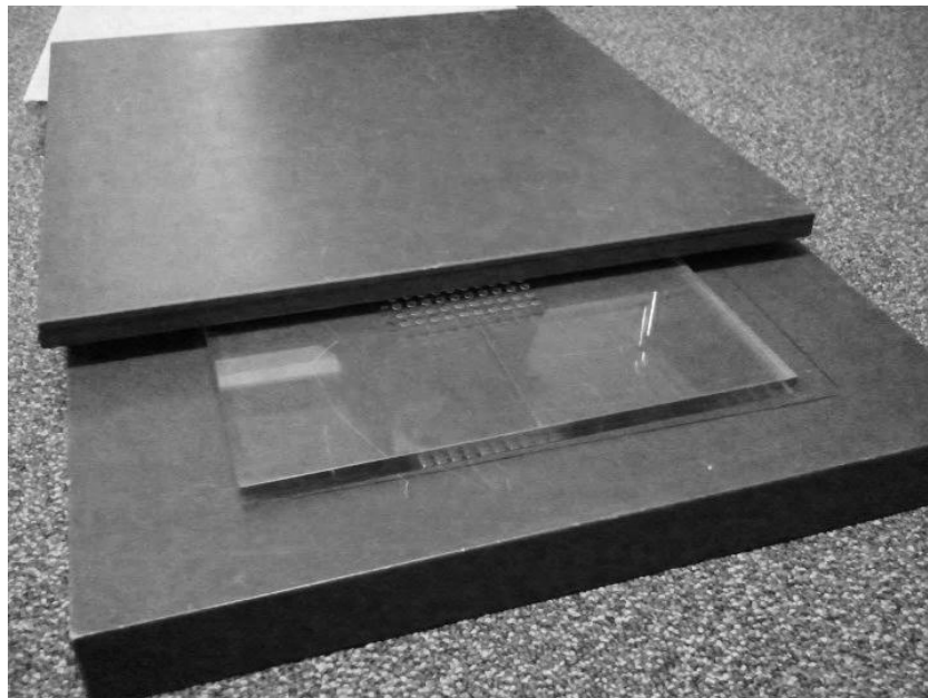
Figure 3. Solid water material (brown) and TLD PMMA template.
