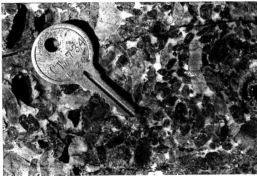
Plate 11. The selective replacement of magnesite conglomerate by chert.
