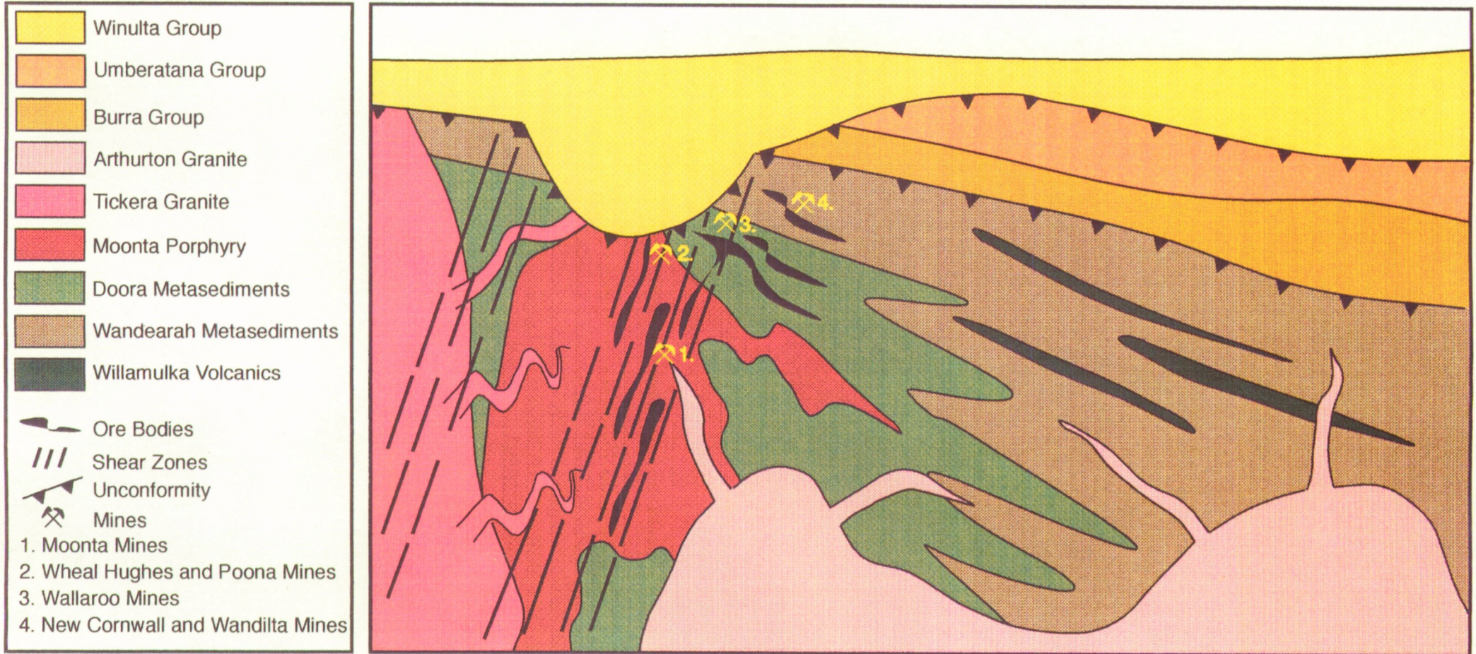
Figure 2.4: Rock relationship diagram showing recognised lithologies in the Moonta Sub-domain and relationship of shears and lithologies to the mineralisation.
