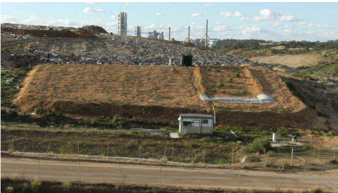
Figure 4.33 Completed Test Sections with Lysimeter (right) and Control (left) Sections. (Photo courtesy of IW Projects (2010))
