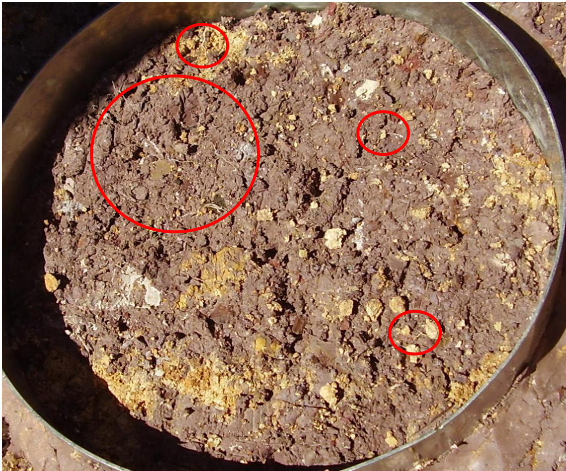
Figure 7.9 Fine Roots (circled) Growing in the Clay Barrier in December 2008
