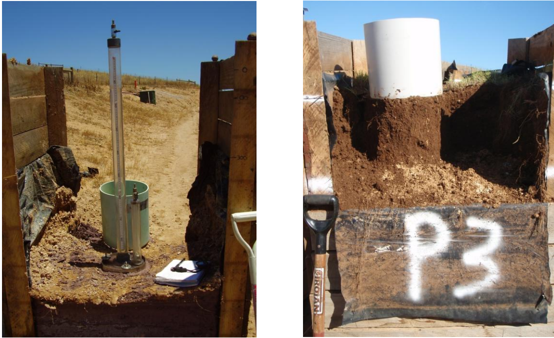
Figure 7.3 CSIRO Disc Permeameter (left) and Removing Undisturbed Core (right) from Box Trial
