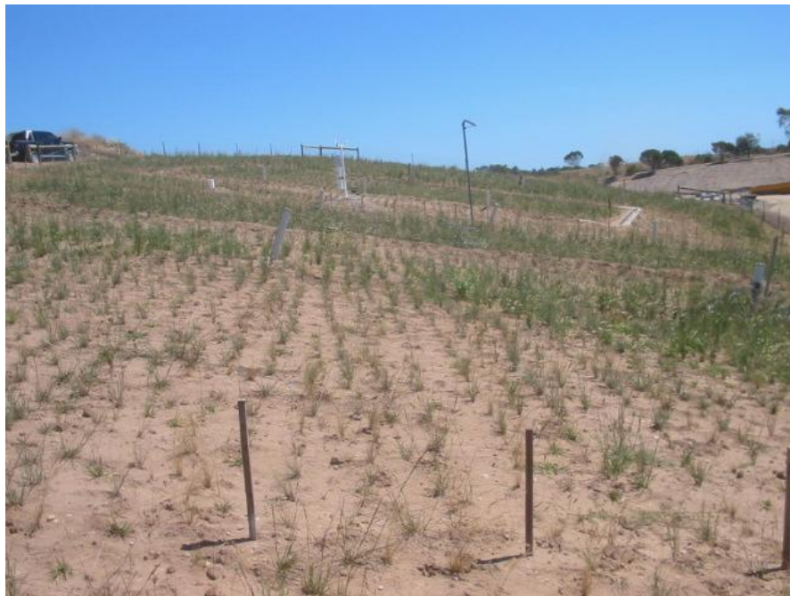
Figure 4.11 SWD Trial Site with Phytocap in the Foreground and Conventional Cover in the Background (November, 2007)
