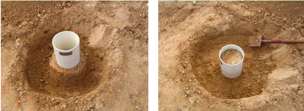
Figure 3.7 Trenching for Undisturbed Soil Sample Collection (left) and Pipe Slid Over Core Sample (right)
