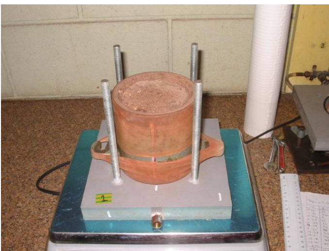
Figure 7.1 Laboratory Trial Recompacted Soil Core and Permeability Apparatus
