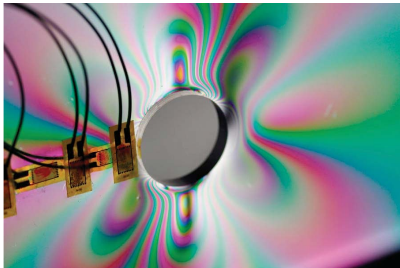
Figure 2.2. Photoelastic fringe pattern of a polycarbonate plate with a hole, loaded uniformly (Fiene 2010).
