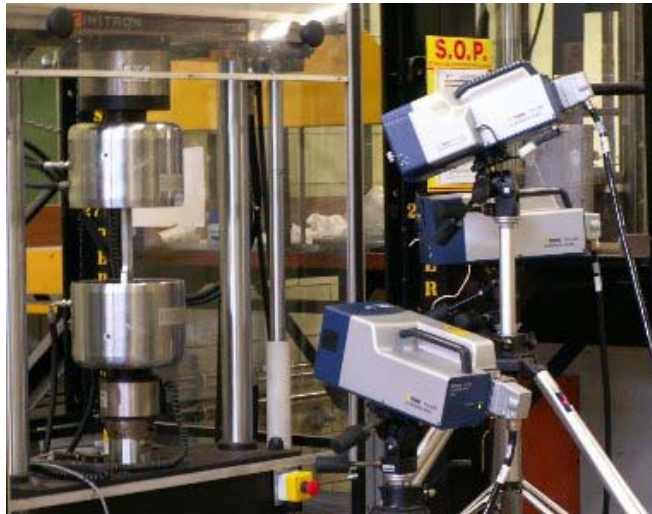
Figure 4.3. Photograph of the 3D vibrometer focused at an aluminium dogbone specimen clamped in an Instron 1342 hydraulic test machine (Cazzolato et al. 2008).
