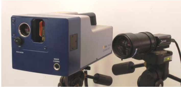
Figure 3.2. Photograph of the 1D vibrometer mounted on a tripod, along with external high-resolution video camera.
