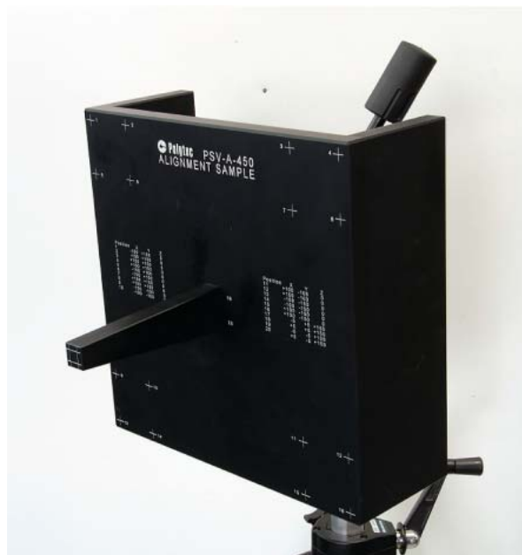
Figure 3.5. Three-Dimensional Alignment Specimen (PSV-A-450).
