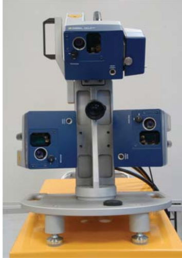
Figure 3.4. 3D vibrometer (PSV-400-3D) mounted on a fix support (PSV-A-T34).
