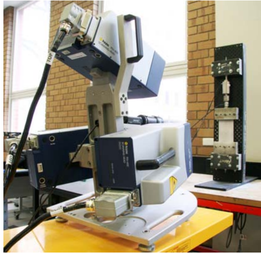
Figure 3.12. Experimental setup of in-plane measurement experiments.
