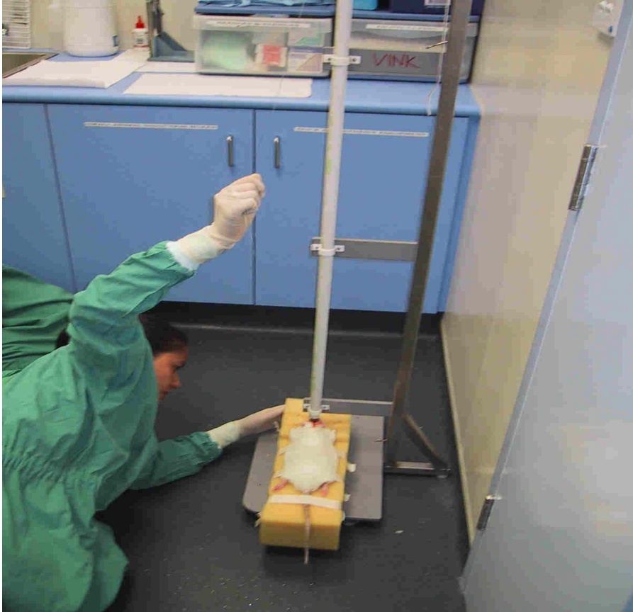
Figure 2.1. The impact acceleration weight drop model. Note that the weight was carefully aligned to centrally strike the steel disc attached to the animal's skull. The animal was fixed to the foam bed using adhesive tape.
