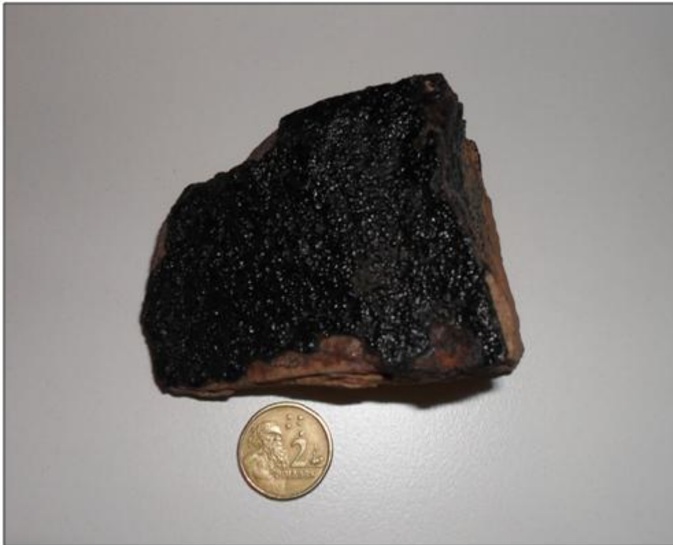
Appendix 33: Iron cementation on fracture surface of Arcoona Quartzite, in faulted region. Located at 0715115 mE 6627901 mN.
