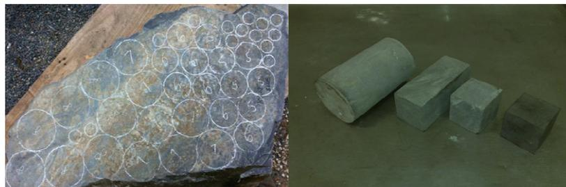
Figure 4.26 Block of Kanmantoo Blue stone and preparation of cubic specimens [after Dong et al., (2011)]
