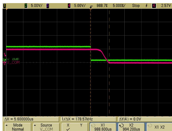
Figure 6.13: Schmitt Trigger falling delay measurement
