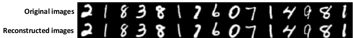
Figure 5.10: The first row represents the original MNIST digits images. The bottom row are the reconstructed images from the DBN autoencoder. The images were obtained from MNIST database (Lee et al. 1998).
