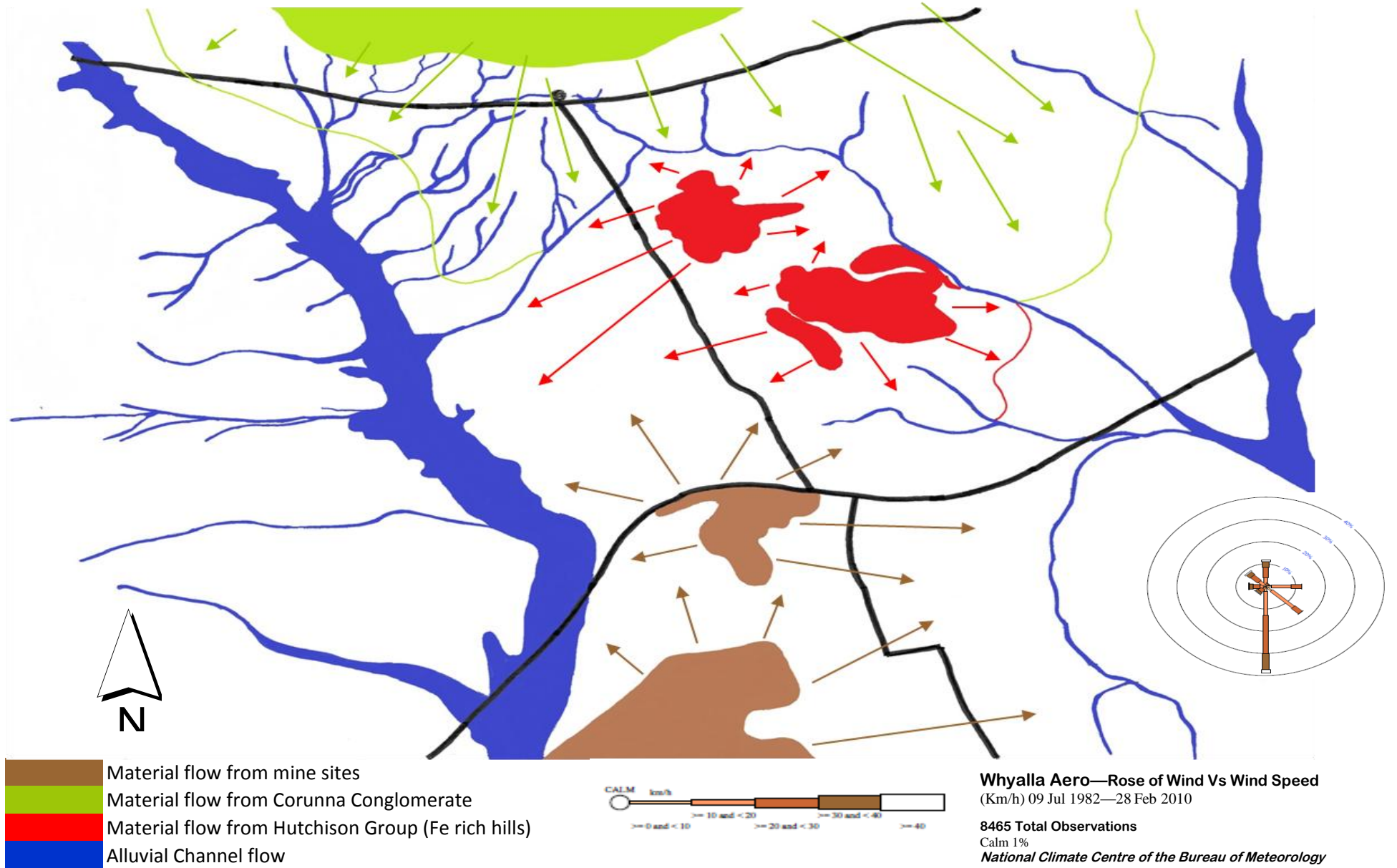
Figure 23: Material Transport Model - Direction of Material Flow
